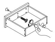
Remove handles from inside drawers using a screwdriver to undo the bolts.
